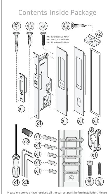
note Euro Lock cylinder supplied separately, specific to the intended door thickness.
