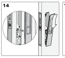
Insert the flush pull with the slide lock into cavity on the chosen side of the door. Push in and down so it grips onto the bottom bracket or edge. Ensure Spindle is inserted through the brass locking slide bar.
