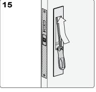
Use Mardeco hex tool to tighten grub screw inside top of flush pull. Ensure it is fitted firmly.
