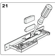
Using a flat screw driver remove the metal backing plate holding the rubber insert in place. Remove the rubber insert and slide the metal plate back in place. Reassemble the assembly plate and 6 screws.
