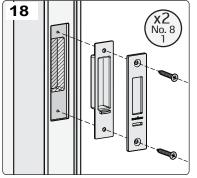
Insert striker plate assembly and secure with two No.8 1 screws.
