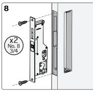
Insert the Euro Lock assembly and secure with two No.8 3/4screws. \*Important \* Refer to step 20/21 before fitting lock.
