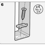
For wooden doors: install two woodfix brackets at top and bottom of cutout on the interior side of the door.
