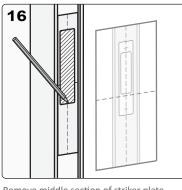
Remove middle section of striker plate template and mark outline for rebate. Use midline as height reference and ensure it lines up with the door. Cut a 4mm rebate.
