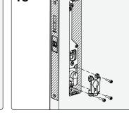
Secure the Euro Lock Cylinder in place with mounting bracket and 3 screws.
