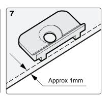
Fix brackets in centre of the cutout with the ridge facing outwards. Ensure that they are approx 1mm inside the edge and do not protrude.
