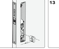
Insert locating pin (Grub Screw) into the Euro Lock cylinder and assemble into the Euro Lock body. Lock Cylinder supplied separately specific to door thickness. Note this is reversible for left/right opening doors.
