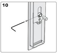
Select the correct spindle size from the guide on the contents page. Add a small amount of the supplied Loctite glue into the spindle hole. Insert spindle and secure with grub screw.
