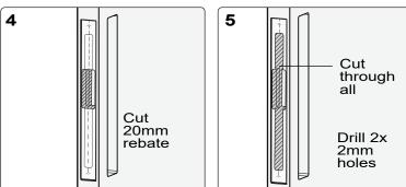
Place middle section of template into rebate and mark second rebate outline. Ensure it is the correct way up. Cut 20mm rebate.
