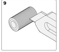
Trim the plastic spacer parts to fit the door thickness. Test fit and retrim if required.
