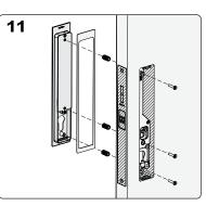
Insert the exterior lock flush pull handle with foam seal (For exterior use only) and trimmed spacer parts and secure with 3 x mounting screws. Refer to contents section for correct screw size
