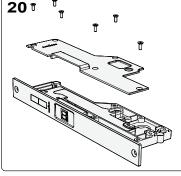
(Optional) Removal of the rubber insert to create a finger pull. Remove the 6 screws holding the assembly plate in place being careful not to remove any internal sliding components.
